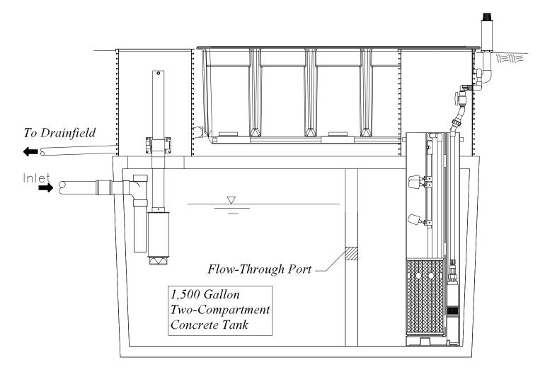
Recirculates through both chambers: Filtrate discharge
