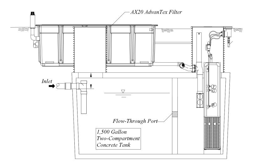
Recirculates through 2<sup>nd</sup> chamber: Filtrate discharge.
